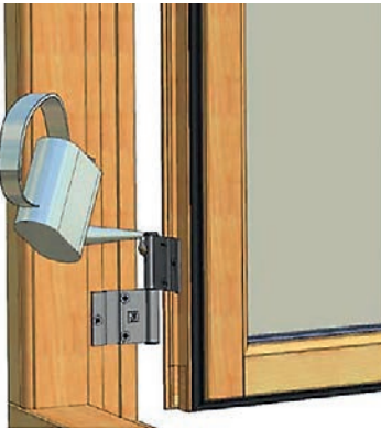
Figure 7.1. Lubricating a butt hinge
