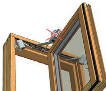
Figure 7.4. Lubricating a side projecting gearing
