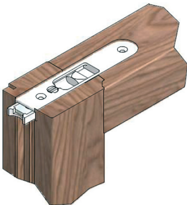
Figure 5.2. Sliding bolts of the bottom sash for a vertical sliding sash window: 1 – open; 2 – closed
