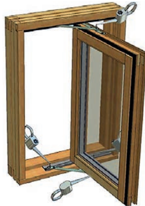
Figure 7.2. Lubricating side projecting gearing
